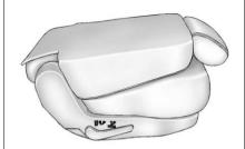
The seatback will fold forward to create a flat load floor.
