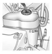
Fill the coolant surge tank with the proper mixture to the FULL COLD mark.
