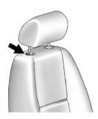
The height of the head restraint can be adjusted. Pull the head restraint up to raise it. Try to move the head restraint to make sure that it is locked in place. To lower the head restraint, press the button, located on the top of the seatback, and push the head restraint down. Try to move the head restraint after the button is released to make sure that it is locked in place.
