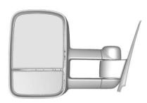
If the vehicle has towing mirrors, they can be adjusted for a clearer view of the objects behind you.
