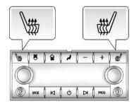
If available, the buttons are on the Rear Seat Audio (RSA) panel on the rear of the center console.
