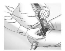
If the belt stops before it reaches the buckle, for lap-shoulder belts with cinching latch plates, tilt the latch plate and keep pulling the safety belt until it can be buckled.
