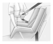
4. For passenger seating positions with a lap-shoulder belt and a free-falling latch plate, pull the rest of the shoulder belt all the way out of the retractor to set the lock. When installing a child restraint using a lap-shoulder belt and a cinching latch plate, skip Step 4 and proceed to Step 5.
