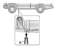
Front Tire Flat: If the flat tire is on a front tire of the vehicle, use the jack handle and only one jack handle extension. Attach the wheel wrench to the jack handle extension. Attach the jack handle to the jack (A). Position the jack on the frame behind the flat tire where the frame sections overlap. Turn the wheel wrench clockwise to raise the vehicle. Raise the vehicle far enough off the ground so there is enough room for the spare tire to clear the ground.
