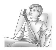
4. Buckle, position, and release the safety belt as described previously in this section. Make sure the shoulder portion of the belt is on the shoulder and not falling off of it. The belt should be close to, but not contacting, the neck. To remove and store the comfort guide, squeeze the belt edges together so that the safety belt can be removed from the guide. Slide the guide onto its storage clip on the interior body.
