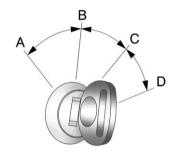
The ignition switch has four different positions.
