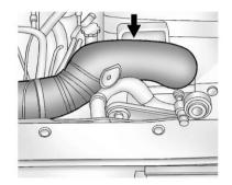
With the coolant surge tank pressure cap off, start the engine and let it run until the upper radiator hose can be felt getting hot. Watch out for the engine cooling fan.
