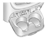
Pull downward on the lid to access the rear floor console cupholders.
