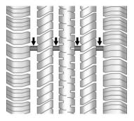
Treadwear indicators are one way to tell when it is time for new tires. Treadwear indicators appear when the tires have only 1.6 mm (1/16 in) or less of tread remaining. Some commercial truck tires may not have treadwear indicators. See *Tire Inspection on page 10-56* and *Tire Rotation on page 10-57* for additional information.
