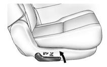
Lift the lever, on the outboard side of the seat, to release the seatback
