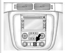
The vehicle may have power assist steps. To enable or disable the power assist steps push ....
