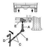
Rear Tire Flat: If the flat tire is on a rear tire of the vehicle, use the jack handle (B) and both jack handle extensions (C). Attach the wheel wrench (D) to the jack handle extensions (C). Attach the jack handle (B) to the jack handle (B) to the jack (A). Use the jacking pad provided on the rear axle. Turn the wheel wrench (D) clockwise to raise the vehicle. Raise the vehicle far enough off the ground so there is enough room for the spare tire to clear the ground.
