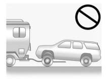
Notice: If a two-wheel drive vehicle or a four-wheel drive vehicle with a single speed automatic transfer case is towed with the rear wheels on the ground, the transmission could be damaged. The repairs would
