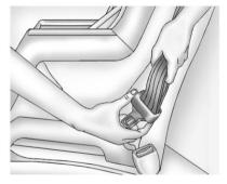
For third row seating positions, with cinching latch plates, tilt the latch plate to adjust the belt if needed.
