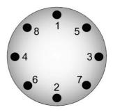
Tighten the nuts firmly in a crisscross sequence as shown by turning the wheel wrench clockwise.
