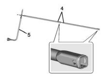
Assemble the two jack handle extensions (4) and wheel wrench (5), as shown.
