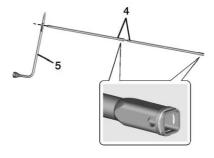
3. Assemble the two jack handle extensions (4) and wheel wrench (5), as shown.
