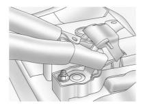
7. Connect the red positive (+) cable to the positive (+) terminal of the vehicle with the dead battery.
