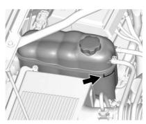
Check to see if coolant is visible in the coolant surge tank. If the coolant inside the coolant surge tank is boiling, wait until it cools down. The coolant level should be at or above the full cold mark. If it is not, there may be a leak in the cooling system.
