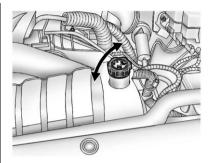
Park the vehicle on a level surface and turn the vehicle off. Remove the DMCM coolant surge tank pressure cap when the DMCM cooling system, including the DMCM coolant surge tank pressure cap and DMCM cooling hoses, are no longer hot. Turn the DMCM coolant surge tank pressure cap slowly counterclockwise (left) about one full turn. Wait 30 seconds.
