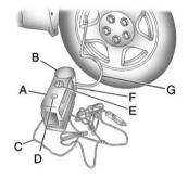
When using the tire sealant and compressor kit during cold temperatures, warm the kit in a heated environment for five minutes. This will help to inflate the tire faster. If a tire goes flat, avoid further tire and wheel damage by driving slowly to a level place. Turn on the hazard warning flashers.
