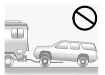
*Notice:* If a two-wheel drive vehicle is towed with the rear wheels on the ground, the transmission could be damaged. The repairs would not be covered by the vehicle warranty. Never tow the vehicle with the rear wheels on the ground.
