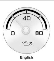
The oil pressure gauge shows the engine oil pressure in psi (pounds per square inch) when the engine is running. Canadian vehicles indicate pressure in kPa (kilopascals). The oil pressure gauge will read zero when operating in the AUTO STOP mode.
