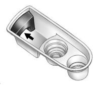
1. Remove the tray by pulling up on the finger depression to access the tire sealant and compressor kit.
