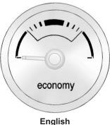
This gauge shows when the vehicle is operating at a fuel efficient point.
