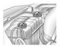
The coolant level should be at or above the FULL COLD mark with the vehicle parked on a level surface. If it is not, there might be a leak at the DMCM cooler core, DMCM pressure cap, DMCM cooler hoses, DMCM cooling pump or somewhere else in the DMCM cooling system. *Notice:* Running the engine when there is a leak in the hybrid cooling system can cause the hybrid cooling system to lose all coolant and can damage the system. Get any leak fixed before you drive the vehicle or run the engine.
