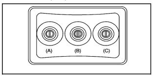
The A/V jacks, located on the rear of the floor console, allow audio or video signals to be connected from an auxiliary device such as a camcorder or a video game unit to the RSE system. Adapter connectors or cables (not included) might be required to connect the auxiliary device to the A/V jacks. Refer to the manufacturer's instructions for proper usage.
