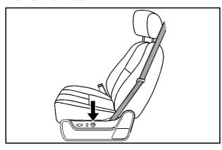
On seats with power lumbar, the controls used to operate this feature are located on the outboard side of the seats.
