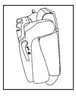
Lift the lever again to release the rear of the seat from the floor. The seat will tumble forward.
