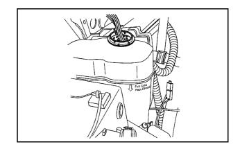
3. Fill the coolant surge tank with the proper mixture to the FULL COLD mark.
