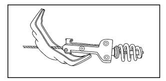
Once the retainer is separated from the guide pin, tilt the retainer and pull it through the center of the wheel along with the cable and latch.
