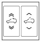
There are two sunroof switches located in the overhead console above the rearview mirror. **Express-Open/Express-Close:** To express-open the sunroof, fully press and release the rear of the driver side switch until the sunroof reaches the desired position. To express-close the sunroof, fully press and release the front of the driver side switch. Press the switch again to stop it.
