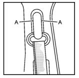
Squeeze the buttons (A) on the sides of the height adjuster and move the height adjuster to the desired position.
