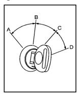
The ignition switch has four different positions.
