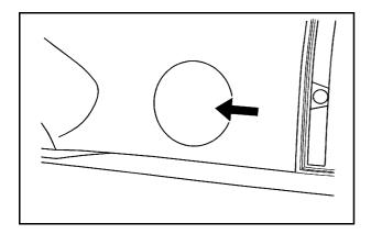
To open the fuel door, push the rearward center edge in and release and it will open.
