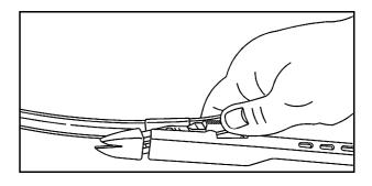
Install the new blade onto the arm connector and make sure the grooved areas are fully set in the locked position.
