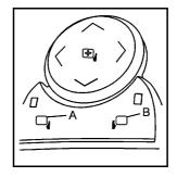
Vehicles with outside power mirrors have the controls on the driver door armrest.
