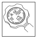
You can remove the coolant surge tank pressure cap when the cooling system, including the coolant surge tank pressure cap and upper radiator hose, is no longer hot.
