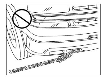
Notice: Never use recovery hooks to tow the vehicle. Your vehicle could be damaged and it would not be covered by warranty.
