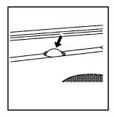
The solar sensor, located in the defrost grille in the middle of the instrument panel, monitors the solar heat. Do not cover the solar sensor or the system will not work properly.
