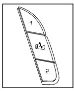
The controls for this feature are located on the driver door, and are used to program and recall memory settings for the driver seat, outside mirrors, and the adjustable throttle and brake pedal feature.
