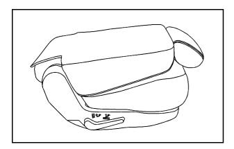
The seatback will fold forward. Leaving the seatback in this position creates a flat load floor.
