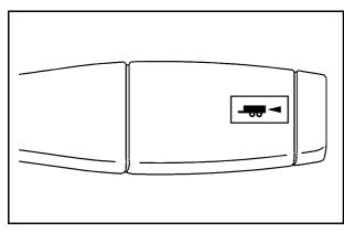
The vehicle has a Tow/Haul mode. The selector button is located on the end of the column shift lever. You can use this feature to assist when towing or hauling a heavy load or if there is a need to charge a battery installed in a trailer. See *Towing a Trailer on page 5-47* for more information.
