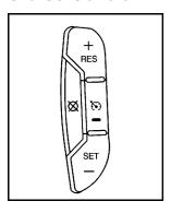
The cruise control buttons are located on left side of the steering wheel.
