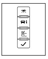
The buttons are the trip/ fuel, vehicle information, customization, and set/ reset buttons. The button functions are detailed in the following pages.
