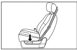
If the seats have power reclining seatbacks, the control used to recline them is located on the outboard side of the seat behind the power seat control.
