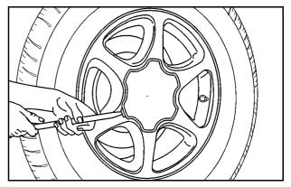
If your vehicle has a center cap that covers the wheel fasteners, place the chisel end of the wheel wrench in the slot on the wheel and gently pry the cap out. If the wheel has a bolt-on hub cap, loosen the plastic nut caps by turning the wheel wrench counterclockwise. The plastic nut caps will be retained in the hub cap after it is removed from the wheel.
