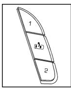
The controls for this feature are located on the driver's door panel, and are used to program and recall memory settings for the driver's seat, outside mirrors, and the adjustable throttle and brake pedal.
