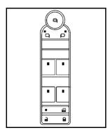
The power window switches are located on the driver door. In addition, each passenger door has a switch for its own window.
