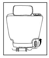
Lift the release lever, located on the bottom rear of the seatback on the outboard side of the seat, and the seatback will fold forward.
