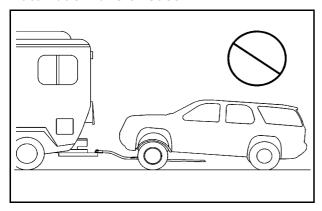
Notice: If a two-wheel drive vehicle or a four-wheel drive vehicle with a single speed automatic transfer case is towed with the rear wheels on the ground,
