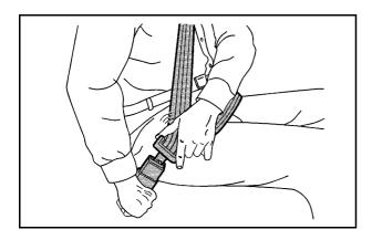
Push the latch plate into the buckle until it clicks. If you find that the latch plate will not go fully into the buckle, see if you are using the correct buckle.
