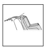
If the position you are using does not have a headrest or head restraint and you are using a dual tether, route the tether over the seatback.
