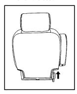
2. Lift the lever, located on the bottom rear of the second row seat on the inboard side, to release the seatback. The seatback will fold forward.
