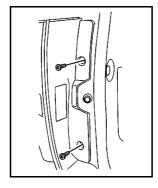
Remove the two screws from the taillamp assembly.
