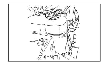
The coolant surge tank is located in the engine compartment on the passenger side of the vehicle. See *Engine Compartment Overview on page 6-16* for more information on location.
