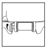
Unlatch the seat from the floor by lifting the lever located next to the carrying handle on the rear of the seat near the bottom.
