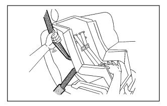
6. To tighten the belt, push down on the child restraint, pull the shoulder portion of the belt to tighten the lap portion of the belt and feed the shoulder belt back into the retractor.
