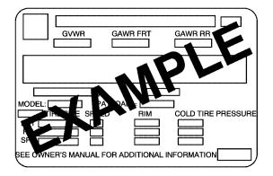
A vehicle specific Certification/Tire label is found on the rear edge of the driver's door. The label shows the size of your vehicle's original tires and the inflation pressures needed to obtain the gross weight capacity of your vehicle. This is called Gross Vehicle Weight Rating (GVWR). The GVWR includes the weight of the vehicle, all occupants, fuel, and cargo.
