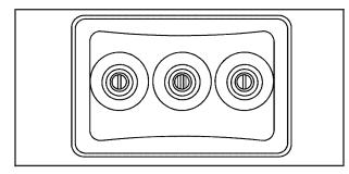
The A/V jacks are located on the rear of the floor console. The A/V jacks allow audio or video signals to be connected from an auxiliary device such as a camcorder or a video game unit to the RSE system. Adapter connectors or cables may be required to connect the auxiliary device to the A/V jacks. Refer to the manufacturer's instructions for proper usage.
