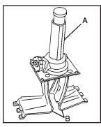
Place the bottom edge of the jack (A) on the wheel blocks (B), separating them so that the jack is balanced securely.
