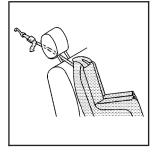
If the position you are using has an adjustable head rest/restraint and you are using a single tether, raise the head rest/restraint and route the tether under the head rest/restraint and in between the head rest/restraint posts.
