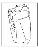
3. Lift the same lever again to release the rear of the seat from the floor. The seat will tumble forward.
