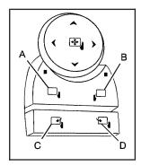
If your vehicle is equipped with outside power foldaway mirrors, the controls are located on the driver's door armrest.
