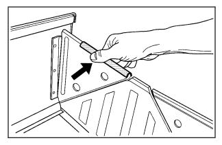
Slide the hinge covers to the center of each side. This will keep the sides of the storage system stationary and allow it to stay upright. Inside the system are two removable dividers. To remove, unhook the loops at the ends of each divider. When not in use, slide the hinge covers back and the storage system will fold back down. Press down on the storage cover to lock it into place.
