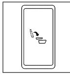
2. Press the automatic seat release button located on the panel behind the rear doors.
