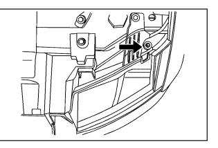
7. Locate the vertical headlamp aiming screws, which are under the hood near each headlamp assembly.
