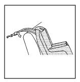
If the position you are using does not have a head rest/restraint and you are using a dual tether, route the tether over the seatback.
