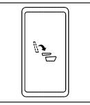
2. Press the automatic seat release button located on the panel behind the rear doors.
