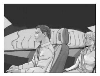
If your vehicle has a roof-mounted rollover airbag for the right front passenger and the person directly behind that passenger, it is located in the ceiling above the side windows.
