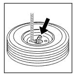
2. Tilt the retainer downward and through the wheel opening. Make sure the retainer is fully seated across the underside of the wheel.
