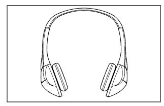
The RSE includes two 2-channel wireless headphones that are dedicated to this system. These headphones are used to listen to media such as CDs, DVDs, MP3s, DVDAs, radio, or any auxiliary source connected to the auxiliary input jack, if your vehicle has this feature or A/V jacks. The wireless headphones have an On/Off button channel 1/2 switch, and a volume control. If your vehicle has a third row video screen display, it will have two additional headphones.
