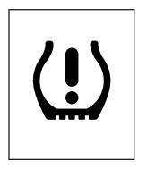
This light will come on briefly when you turn the ignition to RUN. If equipped, a CHECK TIRE PRESSURE DIC message will accompany the light.
