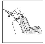
If the position you are using has an adjustable head rest/restraint and you are using a dual tether, route the tether around the head rest/restraint.
