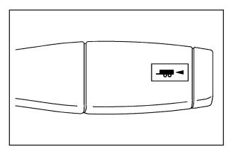
Press this button at the end of the shift lever to enable/disable the tow/haul mode.
