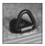
Your vehicle may be equipped with cargo tie downs in the rear cargo area that allow you to strap cargo in and keep it from moving inside the vehicle. **Cargo Management System**
