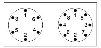
10. Tighten the nuts firmly in a crisscross sequence as shown by turning the wheel wrench clockwise.
