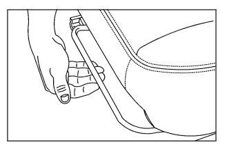
If your vehicle has a manual bucket or a split bench seat, you can adjust the seat forward or rearward with the bar located under the front of the seat cushion.
