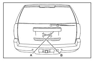
To open the liftglass, press the button on the underside of the license pocket applique (A). The liftglass can also be opened by pressing the liftglass release button on the RKE. To open the entire liftgate, press the touchpad on the underside of the liftgate handle (B). The vehicle must be in PARK (P) to open the liftgate. To close the liftgate, use the pull cup or pull strap as an aid.
