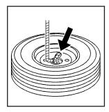
15. Tilt the tire retainer at the end of the cable and pull it through the wheel opening. Pull the tire out from under the vehicle.
