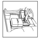
6. Connect the red positive (+) cable to the positive (+) terminal of the vehicle with the dead battery. Use a remote positive (+) terminal if the vehicle has one.
