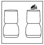
Third Row — Two Passenger (Top Tether Anchor): Seating positions with top tether anchors.
