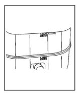
Look at the brake fluid reservoir. The fluid level should be above MIN. If it is not, have your brake system checked to see if there is a leak.
