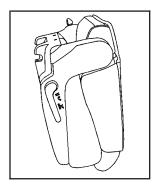
Lift the lever again to release the rear of the seat from the floor. The seat will tumble forward.
