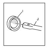
4. Insert the open end of the extension (J) through the hole in the rear bumper (I) (hoist shaft access hole).
