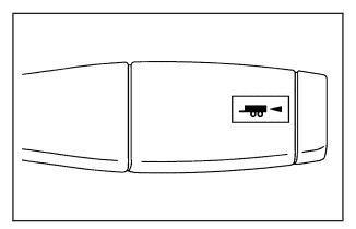
Your vehicle has a Tow/Haul mode. The selector button is located on the end of the column shift lever. You can use this feature to assist when towing or hauling a heavy load or if there is a need to charge a battery installed in a trailer. See *Towing a Trailer on page 416* for more information.
