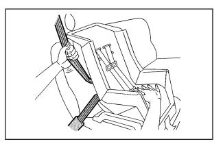
5. To tighten the belt, push down on the child restraint, pull the shoulder portion of the belt to tighten the lap portion of the belt and feed the shoulder belt back into the retractor. If you are using a forward-facing child restraint, you may find it helpful to use your knee to push down on the child restraint as you tighten the belt.
