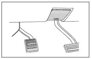
To release the parking brake, hold the regular brake pedal down. Pull the bottom edge of the lever, located above the parking brake pedal, with the parking brake symbol, to release the parking brake. If the ignition is on when the parking brake is released, the brake system warning light will go off.
