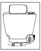
3. Lift the release lever, located on the bottom rear of the seatback on the outboard side of the seat, and the seatback will fold forward.
