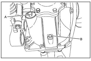
A: Fill Plug B: Drain Plug
