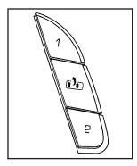
The controls for this feature are located on the driver's door panel, and are used to program and recall memory settings for the driver's seat, outside mirrors, and the adjustable throttle and brake pedal. To save your positions in memory, do the following:
