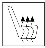
If the rear seats have the heated seat feature, the buttons used to control this feature are located on the Rear Seat Audio (RSA) panel. (Heated Seat): To heat the seat cushion, press the button with the heated seat symbol.
