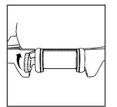
4. Unlatch the seat from the floor by lifting the lever located next to the carrying handle on the rear of the seat near the bottom.
