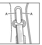
To move it down, squeeze the buttons (A) on the sides of the height adjuster and move the height adjuster to the desired position.
