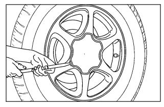
Remove the center cap, if your vehicle has one, by placing the chisel end of the wheel wrench in the slot on the wheel and gently pry the cap out. If the wheel has bolt-on wheel covers, loosen the plastic nut caps by turning the wheel wrench counterclockwise. If needed, finish loosening them by hand. The nut caps will not come off. Using the flat end of the wheel wrench, pry along the edge of the cover until it comes off.
