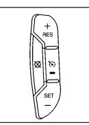
The cruise control buttons are located on left side of the steering wheel. (On/Off): This button can both activate and turn off the system. The indicator light is on when cruise control is on and turns off when cruise control is off.
