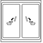
2. From the front seats, press one of the automatic seat release buttons located on the overhead console.
