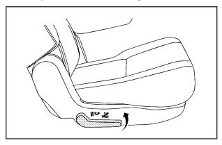
2. Lift the lever, located on the outboard side of the seat, to release the seatback.
