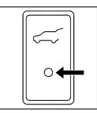
To change the liftgate to manual operation, toggle the switch on the overhead console to the "Disable" position indicated by a circle.
