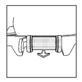
3. Unlatch the seat from the floor by pulling the carrying handle, located at the rear of the seat, rearward.
