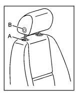
Pull the head restraint up to raise it. To lower the head restraint, press the release button (A), located on the top of the seatback, while you push the head restraint down.
